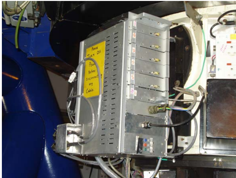
Figure 22: The UNICS hardware, named Common Control Unit (CCU), mounted on IUCAA telescope
